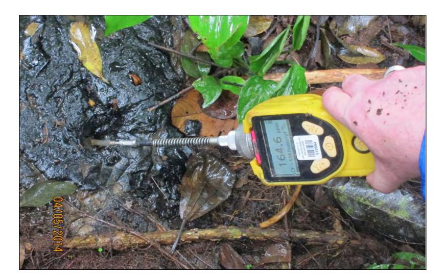
Oil contaminated soil and PID measurement of volatile organic vapors (21.6 ppm) indicative of oil contamination emanating from soil in the seep area at AG-06
