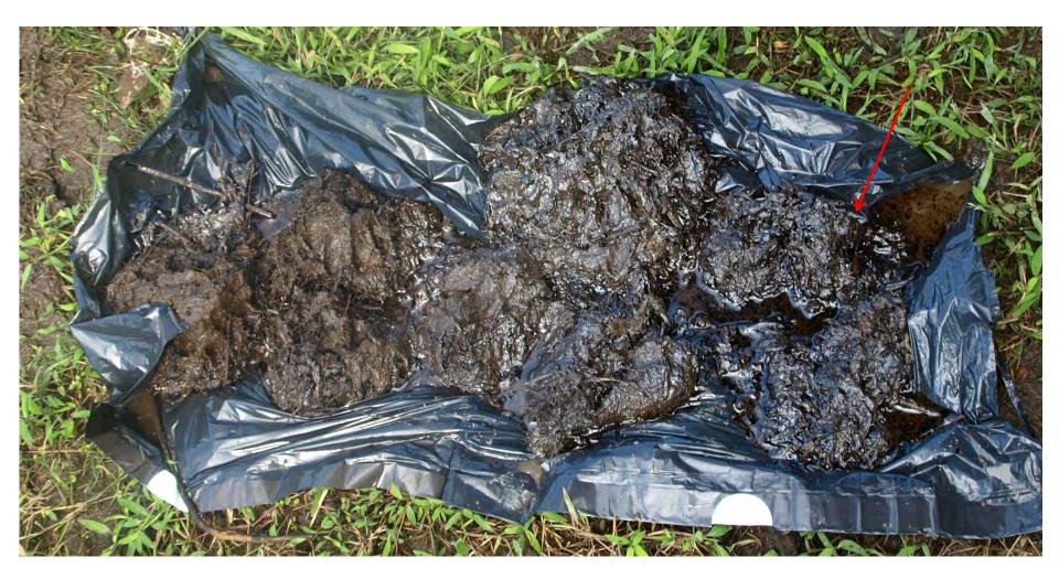
Oil droplets in hand-auger sample of clay from a wetland at YU-02
