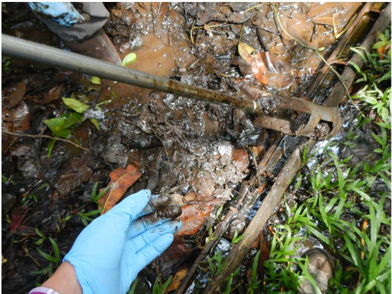
Collecting oil contaminated sediment from stream at SSF-25, note sheens and oil droplets
