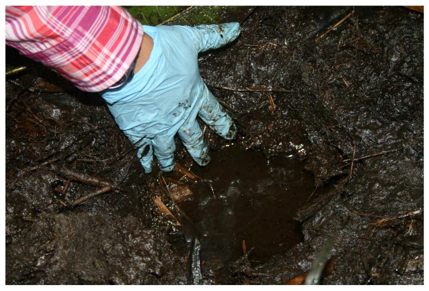
Oil sheen on sediment and groundwater seep at LA-02 with PID reading (10.7 ppm)
